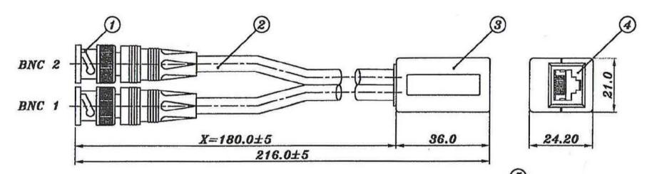
\*Data Rates to 2.048 Mbps \*Speed Ranges 2-8 Mbit/s \*76 Ohm Dual Coax to 120 Ohm Twisted Pair \*Bi-Directional Signal Conversion \*No AC Power or Batteries Needed \*Fenale Coax BNC Connectors Available
