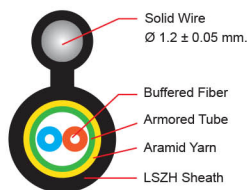
FTTH ROUND, ARMORED, STRANDED DROP CABLE
