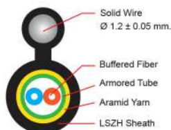
FTTH ROUND, ARMORED, STRANDED DROP CABLE
